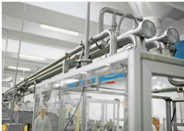
LINEE TRASPORTO BURRO A CIRCUITO CHIUSO CLOSED CIRCUIT BUTTER CONVEYOR LINES
